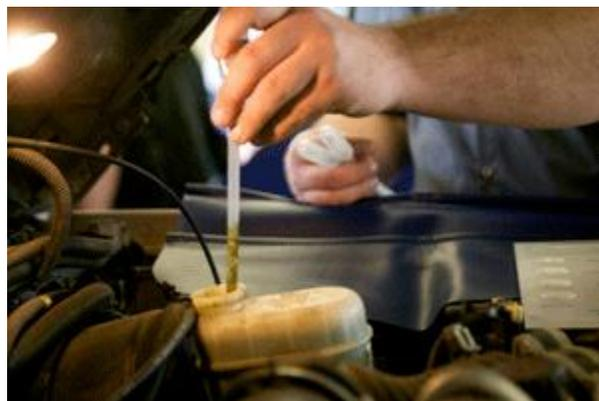
A technician takes a sample of brake fluid for testing. In many cases, radial planar chromatographic tests can quickly and easily tell if a lubricant or fluid needs to be replaced.
