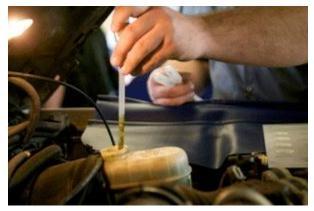
A technician takes a sample of brake fluid for testing. In many cases, radial planar chromatographic tests can quickly and easily tell if a lubricant or fluid needs to be replaced. applying a small fluid sample to a piece of paper.
